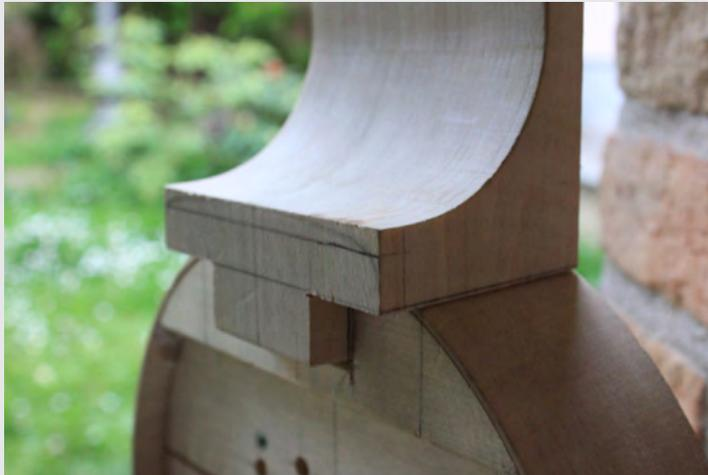
Preparation, gluing and dowelling of the neck, lower belly
